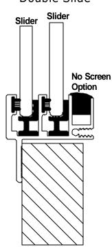
The Series 1200 is a clamp ring window designed specifically for marine applications. It offers customers the choice of forward (front to rear), rear (rear to front) or double-sliding glass configurations. A unique high-back slider track design and ample face slots give the Series 1200 quick water evacuation and excellent slide capability in the most severe conditions.
