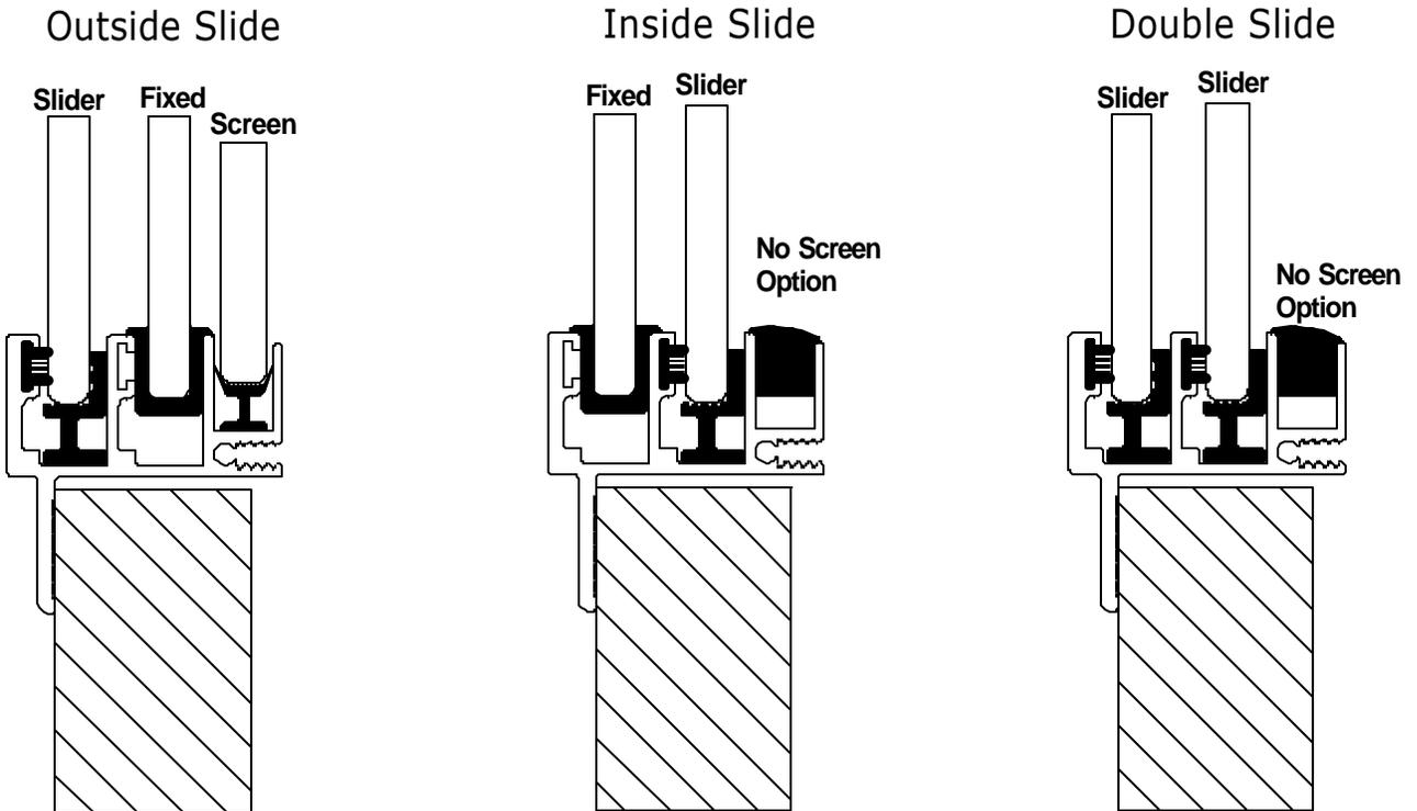
The Series 1260 is a clamp ring window designed specifically for marine applications. It offers customers the choice of forward (front to rear), rear (rear to front) or double-sliding glass configurations. A unique high-back slider track design and ample face slots give the Series 1260 quick water evacuation and excellent slide capability in the most severe conditions.
