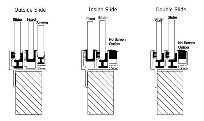
The Series 1260 is a clamp ring window designed specifically for marine applications. It offers customers the choice of forward (front to rear), rear (rear to front) or double-sliding glass configurations. A unique high -back slider track design and ample face slots give the Series 1260 quick water evacuation and excellent slide capability in the most severe conditions.
